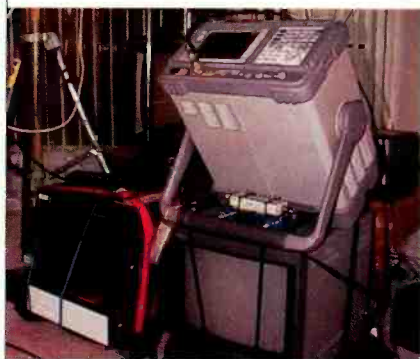
Sinclair's comparison test of 8-VSB and COFDM used indoor antennas and American and European set-top boxes. The tests wrap up this week, as the European COFDM gear is needed for DTV trials in Brazil.
